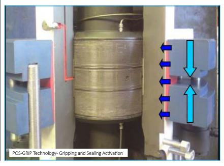
The process is accurately controlled by hydraulic pressure and occurs within the elastic limits of the material, so that the connection is reversible which has many advantages including facilitating side tracking and delivering further savings on decommissioning.
