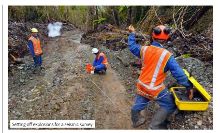
using explosives or thumper trucks to slam heavy plates
